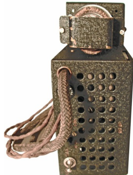
Front panel view of BP series AC mains power unit.
