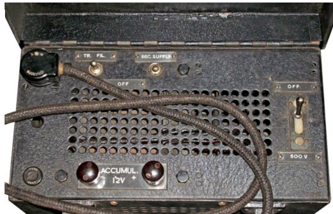
500V Converter Unit with English inscriptions and a slightly different construction. Note the different position of the four hex bolts compared to the illustration top left, indicating a different type of rotary converter.
